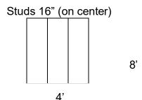
Type 2 – The mock-up shall consist of a minimum of one eight foot wide (2400 mm) by four foot high (1200 mm) sheet of plywood, OSB or drywall that has wood or metal framing on one side. The framing side shall have stude spaced at 24 inches (600mm). See diagram. The other side of the sheathing can be left open to simulate an exterior wall application. The candidate shall spray both sides of the mock-up wall for the Field Examination to simulate interior installation and exterior installations.
