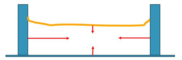
The negative pressure puts a stress on each cell and the foam wants to shrink to equalize the pressure inside the cell (foam) with the pressure outside the cell (foam).
