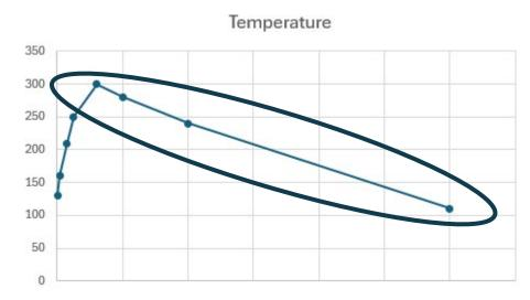
Cellular polymer cools over a period of time but the size of the cell is fixed when it was at a high temperature.
