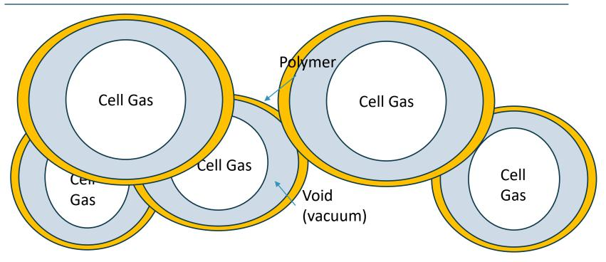
After cooling, we have a slightly negative pressure in the cells because the polymer was a "fixed" size when it was created **at the higher temperature**.
