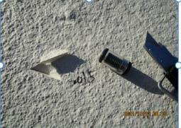
View of slit sample taken from the section that had base coating application applied.
