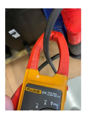
When using amp clamp meter, always run power wire through the clamp and, NOT clamped onto the wire.
