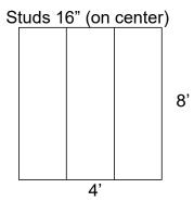
Type 2 – The mock-up shall consist of a minimum of one eight foot wide (2400 mm) by four foot high (1200 mm) sheet of plywood, OSB or drywall that has wood or metal framing on one side. The framing side shall have stude spaced at 24 inches (600mm). See diagram. The other side of the sheathing can be left open to simulate an exterior wall application. The candidate shall spray both sides of the mock-up wall for the Field Examination to simulate interior installation and exterior installations.
